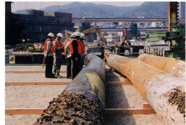
Example of damage to a mooring wharf after the 1995 Hanshin-Awaji Earthquake (The wharf appeared to be sound, but the steel sheet piles had buckled)
